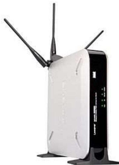
Fig. 7.1 Wireless access point
