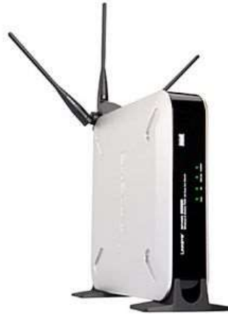
Fig. 7.1 Wireless access point
